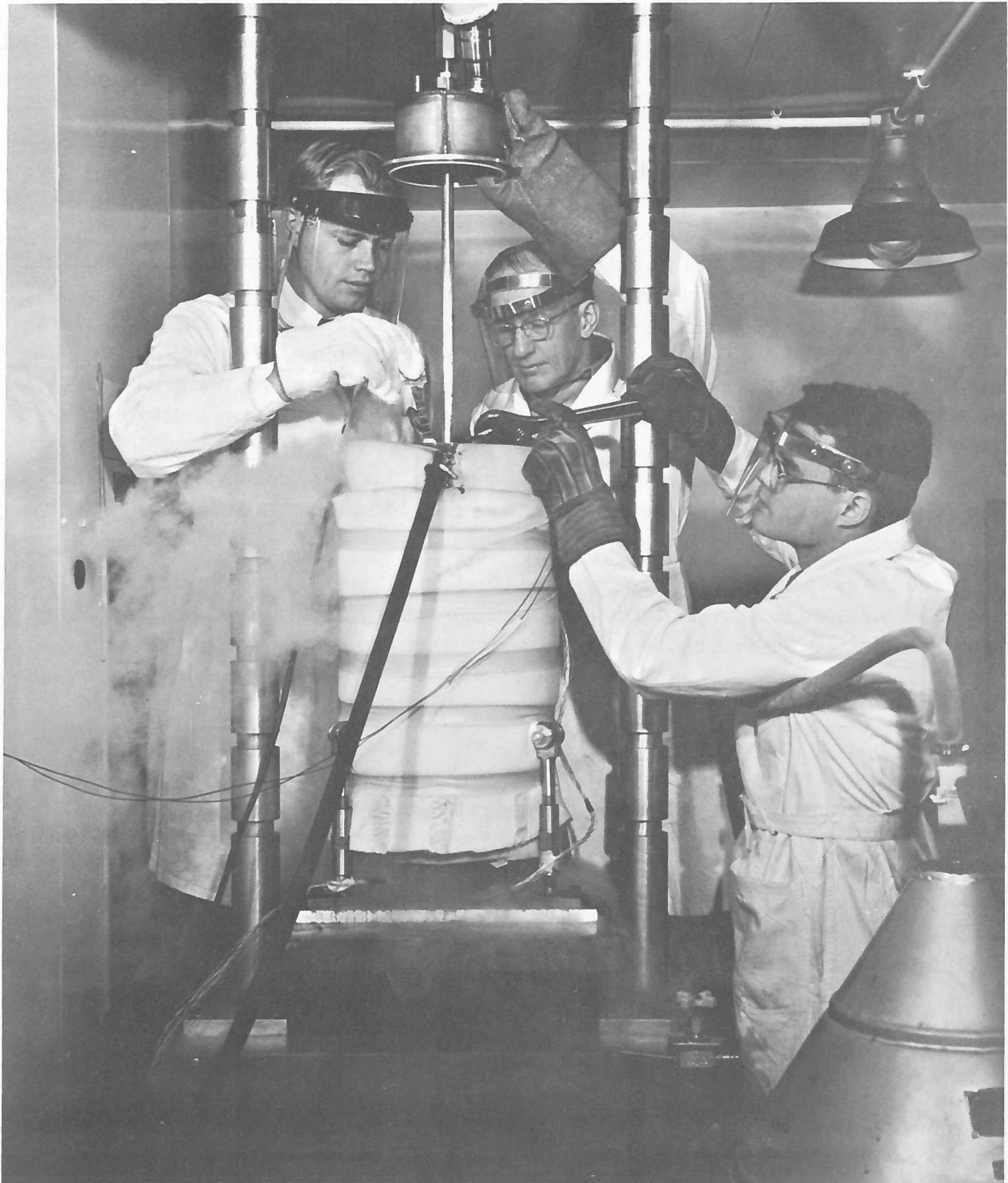
Figure 11. Astronautics' cryogenic tensile testing setup.
