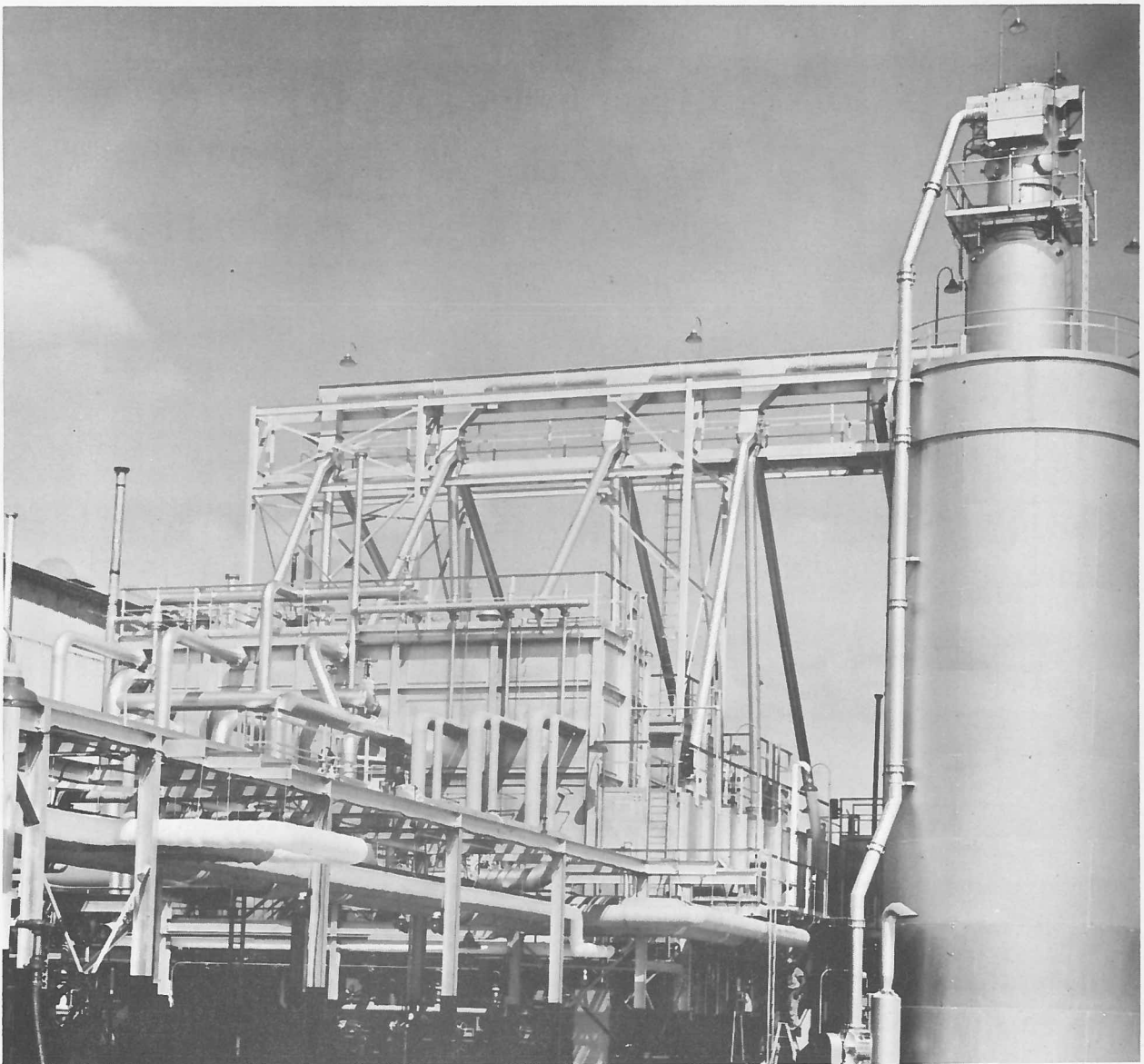
Figure 4. Converter cold box for liquefying hydrogen.
